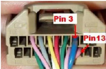
This is the view of the radio connector in the vehicle
