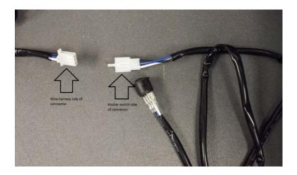
Now plug the HE-WRC receiver box into the white 3 pin connectors of the rocker switch side and the wire harness side. Now you have successfully added wireless control capability to your HEISE lighting. Now secure the HE-WRC receiver box either by screws or wire ties.
