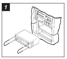
Disconnect the negative battery terminal to prevent an accidental short circuit. Unsnap the side trim pieces from the factory head unit. Using Metra's 86-5618, pull the unit from the dash and disconnect the wiring.
