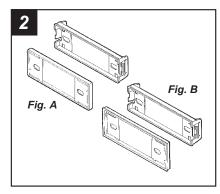
Locate the **Snap-in Bracket** and **Rounded Faceplate** (see Fig. A) OR the **Snap-in Bracket** and **Cornered Faceplate** (see Fig. B). Skip to the Installation Instructions for ALL VEHICLES on Page #21.
