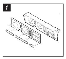
Disconnect the negative battery terminal to prevent an accidental short circuit. Remove (4) Phillips screws from the top edge of the dash trim bezel. Remove the light switch knob, cigarette lighter and ashtray. Unsnap the molding located below the dash trim bezel and remove (4) screws exposed. Remove (4) screws securing the factory head unit and disconnect the wiring.
