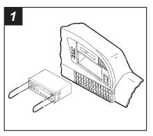
Disconnect the negative battery terminal to prevent an accidental short circuit. Using Metra's **86-5618**, pull the factory head untifrom the dash and disconnect the wiring.
