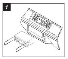
Disconnect the negative battery terminal to prevent an accidental short circuit. Using Metra's **86-5618**, pull the factory head unit from the dash and disconnect the wiring.
