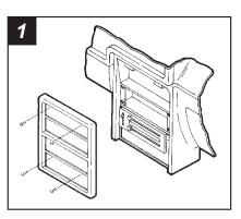
Disconnect the negative battery terminal to prevent an accidental short circuit. Remove (2) screws from the top of the dash trim bezel. Open the ashtray and remove (2) screws from the ashtray cavity. Remove (4) screws securing the factory head unit and
