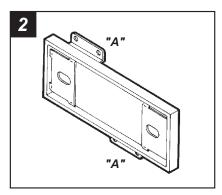
Cut and remove all mounting tabs on the Radio Housing EXCEPT tabs "A". The mounting tabs can be identified by the stamped letter on the back of each tab. Skip to the Installation Instructions for ALL VEHICLES on Page #22.
