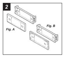
Locate the **Snap-in Bracket** and **Rounded Faceplate** (see Fig. A) OR the **Snap-in Bracket** and **Cornered Faceplate** (see Fig. B). Skip to the Installation Instructions for ALL VEHICLES on Page #21.
