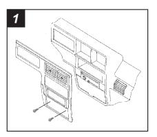
Disconnect the negative battery terminal to prevent an accidental short circuit. Remove the ashtray and (2) screws exposed in the ashtray cavity. Using Metra's 86-5618, pull the factory head unit from the dash and disconnect the wiring.
