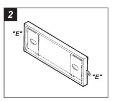
Cut and remove all mounting tabs on the *Radio Housing* EXCEPT tabs *"E"*. The mounting tabs can be identified by the stamped letter on the back of each tab. *Skip to the Installation Instructions for ALL VEHICLES on Page #22*.
