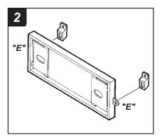
Cut and remove all mounting tabs on the *Radio Housing* EXCEPT tabs "E". The mounting tabs can be identified by the stamped letter on the back of each tab. Locate *Spacer Set #1*. (The Spacers must be placed behind the mounting tabs during installation in step #5). *Skip to the Installation Instructions for ALL VEHICLES on Page #22*.
