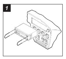
Disconnect the negative battery terminal to prevent an accidental short circuit. Using Metra's **86-5618**, pull the factory head unit from the dash and disconnect the wiring.
