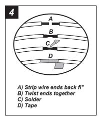
Locate the factory wiring harness in the dash. Metra recommends using the proper mating adaptor and making connections as shown. (Isolate and individually tape off the ends of any unused wires to prevent electrical short circuit).
