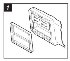
Disconnect the negative battery terminal to prevent an accidental short circuit. Carefully pull and remove the dash trim bezel. Remove (4) screws securing the factory head unit and disconnect the wiring.
