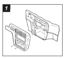
Disconnect the negative battery terminal to prevent an accidental short circuit. Remove (2) screws from the steering column trim panel and (2) screws from the ashtray cavity. Unclip the dash trim bezel. Using Metra's 86-5618, pull the factory head unit unit from the dash and disconnect the wiring.
