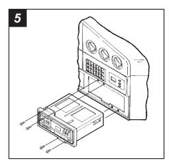
Re-connect the battery terminal and test the unit for proper operation. Mount the head unit/kit assembly to the sub-dash with those screws previously removed.
