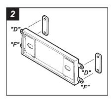
Cut and remove all mounting tabs on the *Radio Housing* EXCEPT tabs "D" and "F". The mounting tabs can be identified by the stamped letter on the back of each tab. Locate *Spacer Set #2*. (The Spacers must be placed behind the mounting tabs during installation in step #5). *Skip to the Installation Instructions for ALL VEHICLES on Page #22*.
