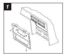
Disconnect the negative battery terminal to prevent an accidental short circuit. Remove (4) screws from the top edge of the dash trim bezel. Remove (2) screws from the bottom edge of the dash trim bezel. Remove the climate control knobs and remove the bezel. Remove (4) hex-head screws securing the factory head unit and disconnect the wiring.
