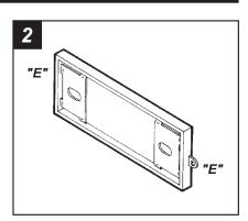
Cut and remove all mounting tabs on the *Radio Housing* EXCEPT tabs "E". The mounting tabs can be identified by the stamped letter on the back of each tab. *Skip to the Installation Instructions for ALL VEHICLES on Page #22.*
