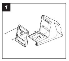
Disconnect the negative battery terminal to prevent an accidental short circuit. Gently remove the climate control trim panel and (2) Phillips screws exposed. Lift up on the dash trim bezel and remove. Remove (2) screws securing the factory head unit and disconnect the wiring.
