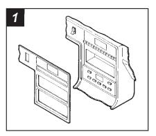
Disconnect the negative battery terminal to prevent an accidental short circuit. Gently pry out on the dash trim bezel and remove. Remove (4) 5mm hex-head sheet metal screws securing the factory head unit and disconnect the wiring.
