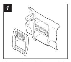
Disconnect the negative battery terminal to prevent an accidental short circuit. Remove (1) screw above the climate controls. Unclip the dash trim bezel. Using Metra's **86-5618**, pull the factory head unit from the dash and disconnect the wiring.
