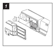
Disconnect the negative battery terminal to prevent an accidental short circuit. Remove (3) torx-head screws from the steering column trim panels. Unscrew the tilt steering lever and unsnap the trim panels. Remove (4) screws from the dash trim bezel and remove the bezel. Remove (2) screws securing the factory head unit and disconnect the wiring.
