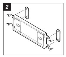
Cut and remove all mounting tabs on the *Radio Housing* EXCEPT tabs "D" and "F". The mounting tabs can be identified by the stamped letter on the back of each tab. Locate *Spacer Set #2*. (The Spacers must be placed behind the mounting tabs during installation in step #5). Skip to the *Installation Instructions for ALL VEHICLES on Page #22*.
