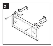
Cut and remove all mounting tabs on the *Radio Housing* EXCEPT tabs "B". The mounting tabs can be identified by the stamped letter on the back of each tab. Mount *Bracket Set #1* to the back of the mounting tabs with (2) #8 x 1" *Phillips screws* supplied. Skip to the Installation Instructions for ALL VEHICLES on Page #22.
