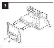
Disconnect the negative battery terminal to prevent an accidental short circuit. Remove the ashtray and (2) screws from the ashtray cavity. Using Metra's **86-5618**, pull the factory head unit from the dash and disconnect the wiring.
