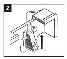
Slide the **Locking Tabs** onto the guides located on the front corners of the **Snap-in Bracket**. Skip to the Installation Instructions for ALL VEHICLES on Page #21.
