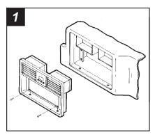
Disconnect the negative battery terminal to prevent an accidental short circuit. Remove (2) Phillips screws from the base of the dash trim bezel. Pry down on the (2) tabs located at the top of the dash trim bezel and remove the bezel. Remove (4) screws securing the factory head unit and disconnect the wiring.
