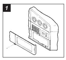
Disconnect the negative battery terminal to prevent an accidental short circuit. Remove (1) 7mm hex-head screw from the bottom of the radio trim bezel. Gently unclip the bezel and disconnect the antenna switch power lead. Remove (4) screws securing the factory head unit and disconnect the wiring.
