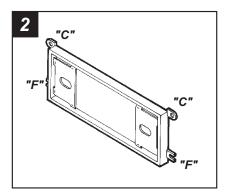
Cut and remove all mounting tabs on the *Radio Housing* EXCEPT tabs "C" and "F". The mounting tabs can be identified by the stamped letter on the back of each tab. *Skip to the Installation Instructions for ALL VEHICLES on Page # 22.*
