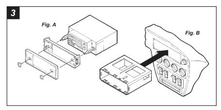
**2-SHAFT HEAD UNITS:** Attach the **Faceplate** to the **Snap-in Bracket**. (If an aftermarket unit with upper-shaft locations is being installed, cut and remove the upper-shaft tabs from the shaft holes in the Snap-in Bracket). Slide the aftermarket head unit into the kit and secure with shaft nuts. (see Fig. A)
