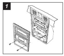
Disconnect the negative battery terminal to prevent an accidental short circuit. Open the ashtray and remove (2) Phillips screws securing the dash trim bezel. Remove (4) screws securing the factory head unit and disconnect the wiring.
