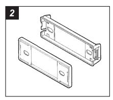
Locate the **Snap-in Bracket** and **Rounded Faceplate**. Skip to the Installation Instructions for ALL VEHICLES on Page #21
