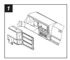
Disconnect the negative battery terminal to prevent an accidental short circuit. Gently unclip the dash trim bezel. Remove (2) screws securing the factory head unit and disconnect the wiring.
