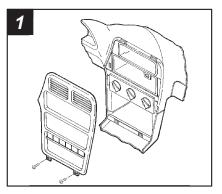
Disconnect the negative battery terminal to prevent an accidental short circuit. Remove (2) screws from the base of the dash trim bezel. Unclip and remove the bezel. Using Metra's 86-5618, pull the factory head unit from the dash and disconnect the wiring.
