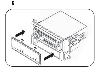
NOTE: To remove the radio unsnap and remove the ISO trim-plate. Using a flat blade screwdriver disengage ISO brackets from the radio housing and slide radio out of radio housing.
