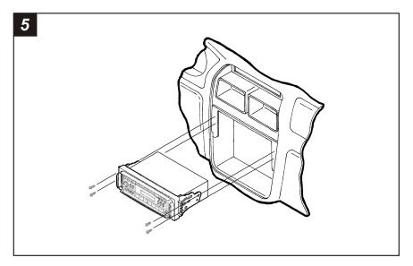
Re-connect the battery terminal and test the unit for proper operation. Mount the head unit/kit assembly to the sub-dash with (4) Phillips screws previously removed in step #1.
