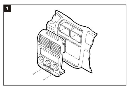
Disconnect the negative battery terminal to prevent an accidental short circuit. Open the cupholder and remove (2) Phillips screws exposed. Lower the glove box and detach the vent cable exposed. Reach under the driver's side dash and detach (2) vent cables located above the accelerator. Unclip the dash trim bezel and remove. Remove (4) screws securing the factory head unit and disconnect the wiring.
