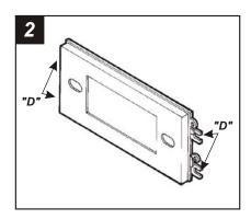
Cut and remove all mounting tabs on *Radio Housing #2* EXCEPT tabs "D". The mounting tabs can be identified by the stamped letter on the back of each tab. *Skip to the Installation Instruc-tions for ALL VEHICLES on Page #5.*
