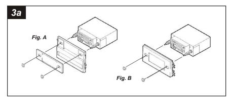
**2-SHAFT HEAD UNITS:** For models using **Radio Housing #1**, attach the **Faceplate** to the Housing. Slide the aftermarket head unit into the kit and secure with shaft nuts. (see Fig. A). For models using **Radio Housing #2**, slide the aftermarket head unit into the kit and secure with shaft nuts. (see Fig. B)
