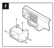
Disconnect the negative battery terminal to prevent an accidental short circuit. Remove (2) screws from each side of the radio trim bezel. Remove the ashtray and (1) screw from the rear support tab. Remove the radio trim bezel/sub-bracket assembly. Remove (4) screws securing the sub-bracket to the back of the radio trim bezel. Loosen (2) screws on top of the bezel and remove the sub-bracket from the bezel.
