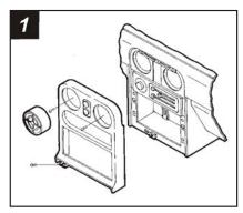
Disconnect the negative battery terminal to prevent an accidental short circuit. Remove (2) screws from the center console storage compartment. Remove (1) screw under the ashtray. Remove (1) screw from each side of the center console panel and remove the panel. Remove (1) screw exposed at the base of the dash trim bezel. Pop out the a/c vents and remove (2) screws exposed. Remove the dash trim bezel.
