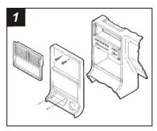
Disconnect the negative battery terminal to prevent an accidental short circuit. Remove the ashtray and (2) screws exposed in the ashtray cavity. Unsnap the gear shifter trim and remove (2) screws exposed. Unsnap the climate control trim bezel and remove (2) screws exposed. Remove the dash trim bezel and disconnect the wiring. Remove (4) screws securing the factory head unit and disconnect the wiring.
