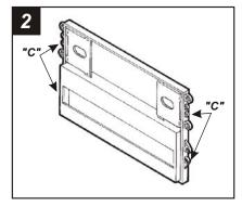
Cut and remove all mounting tabs on *Radio Housing #1* EXCEPT tabs "C". The mounting tabs can be identified by the stamped letter on the back of each tab. *Skip to the Installation Instructions for ALL VEHICLES on Page #5.*
