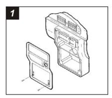
Disconnect the negative battery terminal to prevent an accidental short circuit. Remove the ashtray and (2) screws exposed. Remove the pocket and (2) screws exposed. Remove the radio trim bezel and disconnect the wiring. Remove (4) screws securing the factory dummy plate to the back of the bezel and discard the plate.
