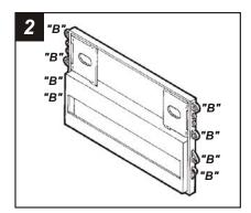
Cut and remove all mounting tabs on *Radio Housing #1* EXCEPT tabs "B". The mounting tabs can be identified by the stamped letter on the back of each tab. *Skip to the Installation Instructions for ALL VEHICLES on Page #5.*
