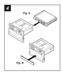
IF AN EQUALIZER WILL BE INCLUDED: Slide the aftermarket equalizer into the back of the Radio Housing. Using the hardware included with the equalizer, mount the unit to the kit. (see Fig. A)
