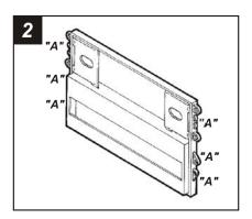
Cut and remove all mounting tabs on *Radio Housing #1* EXCEPT tabs "A". The mounting tabs can be identified by the stamped letter on the back of each tab. *Skip to the Installation Instructions for ALL VEHICLES on Page #5.*
