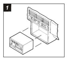
Disconnect the negative battery terminal to prevent an accidental short circuit. Reach behind the console and remove (2) nuts supporting the head unit carrier. Remove the factory head unit and disconnect the wiring..
