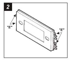
Cut and remove all mounting tabs on *Radio Housing #2* EXCEPT tabs *"E"*. The mounting tabs can be identified by the stamped letter on the back of each tab. *Skip to the Installation Instructions for ALL VEHICLES on Page #5.*
