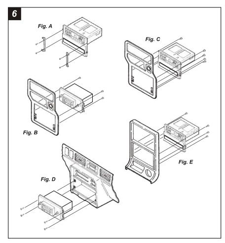
**B-SERIES PICKUP:** Re-connect the battery terminal and test the unit for proper operation. Mount **Bracket Set #1** to the Housing with **(4)** ½" **Hex-head Screws** supplied. Mount the head unit/kit assembly to the back of the dash trim bezel with **(4)** screws removed in step #1 and re-attach the bezel. (see Fig. A)
