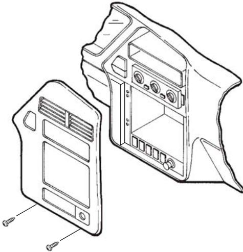
Disconnect the negative battery terminal to prevent an accidental short circuit. Remove (2) screws from the base of the radio trim bezel. Unclip the bottom edge of the radio trim bezel and disconnect the hazard light, defroster, wiper and cigarette lighter wiring. Remove the radio trim bezel. Remove (4) screws securing the factory head unit and disconnect the wiring.
