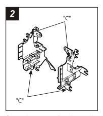
Cut and remove all tabs on the Mounting Brackets EXCEPT tabs "C". (The tabs can be identified by the stamped letter by each tab). Skip to the Installation Instructions for ALL VEHICLES on Page #3.
