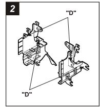
Cut and remove all tabs on the Mounting Brackets EXCEPT tabs "D". (The tabs can be identified by the stamped letter by each tab). Skip to the Installation Instructions for ALL VEHICLES on Page #3.
