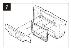
Disconnect the negative battery terminal to prevent an accidental short circuit. Remove the climate control knobs and (2) Phillips screws exposed. Unclip and remove the climate control trim bezel. Depress the side clips securing the climate control panel and move the panel to access (2) Phillips screws from the top of the factory radio brackets. Remove the ashtray. Unclip and remove the radio trim bezel. Remove (2) Phillips screws from the bottom of the radio brackets and disconnect the wiring.
