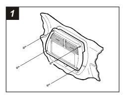
Disconnect the negative battery terminal to prevent an accidental short circuit. Remove (4) 3/16" Allen Screws from the radio trim bezel and remove the bezel. Remove (4) 10mm bolts securing the factory head unit and disconnect the wiring.
