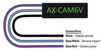
\* Accessory power can also be used if the radio has the option to monitor the camera while in motion
