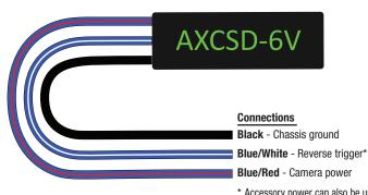
\* Accessory power can also be used if the radio has the option to monitor the camera while in motion
