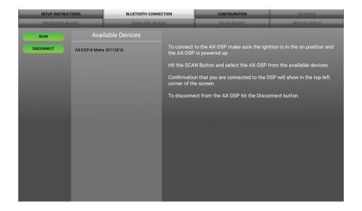
Scan - Press this button to start the Bluetooth pairing process, then select the interface
