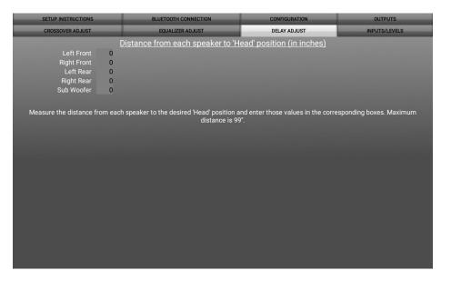
Allows a delay of each channel. If a delay is desired, first measure the
