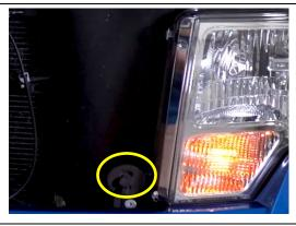
3) Remove the torx bolt behind the stop, place the bracket over the hole, and reinstall the torx bolt.
