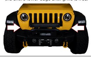
Using supplied hardware, secure the upper grille mounting plate to the grille panel. On both sides of grille.
