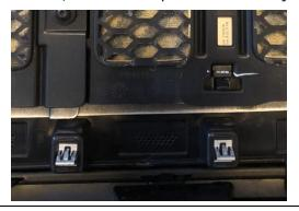
2. Starting at one side of the grille, firmly pull out on the bottom edge to release it from the panel. Continue this process across the entire lower edge until grille is free.
