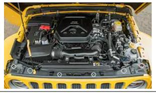
3. Using a flat blade screw driver, remove the factory clips from the Jeep grille. Transfer to JP-GRILLE1, secured to post like factory.
