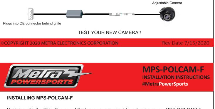
Vehicles with the Ride Command Systems are pre-wired for a front camera. MPS-POLCAM-F plugs directly into the factory connector.
