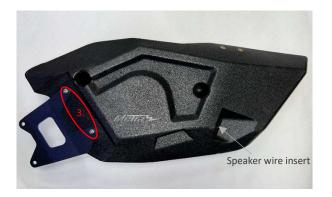
4. Placing door pod, into door frame lining up capture nuts and bracket holes. Using (2) M6x16mm bolts, (4) washers, and (2) nuts.
