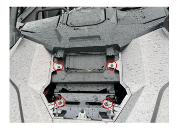
4. Using a soft pry tool, remove the gray trim panels from the dashboard.
