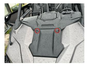
2. Remove two (2) T-40 TORX bolts located under hood holding dash in place.
