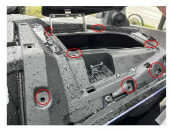
8. Pull up fender panels, but do not detach from chassis. Allow fenders to rest open.
