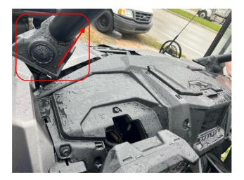
6. Remove (4) T-40 bolts from dash panel on the drivers side of the vehicle.
