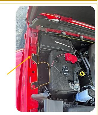
• Install bracket using factory bolt, and supplied M6 bolt. Tighten with 10mm socket/wrench.
