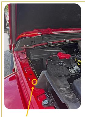
• Remove factory bolt using 10mm socket/wrench
