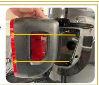
4. Locate OE connector, slide red locking tab back and disconnect.
