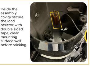
Plug the JP-TL06S into the OE connector and reassemble using the original 8mm bolts.
