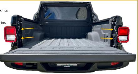
Pull the light assembly straight back releasing the two locating tabs.
