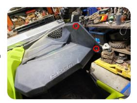
4. Using a flat blade screw driver loosen and the hose clamp and remove the outside panel.
