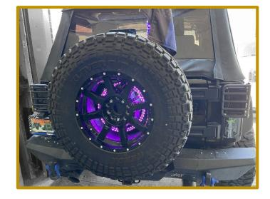
1. Assemble the wheel ring, at the 11" configuration.
