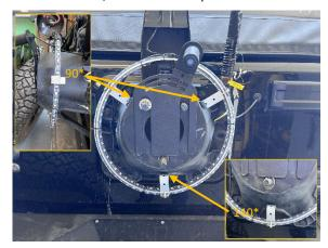
To complete install, connect controller to ring light and remount spare tire.
