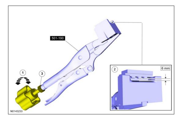
3. Notice: make sure the mirror remover is fully inserted into the interior rear view mirror mount access hole. Otherwise, damage to the windshield glass may occur.
