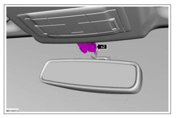
NOTICE: To present damage to the mirror or base, rotate the mirror base with hands only, do not use tools.
