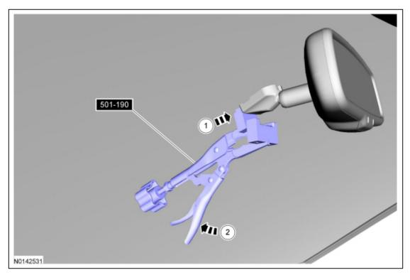
4. Using a closed hand, bump the adjustment handle of the mirror remover to slide the mirror upward on the mirror mount.
