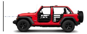
4. To create your X-axis (horizontal) line, make a straight-line using tape by connecting the center points between the headlights.
